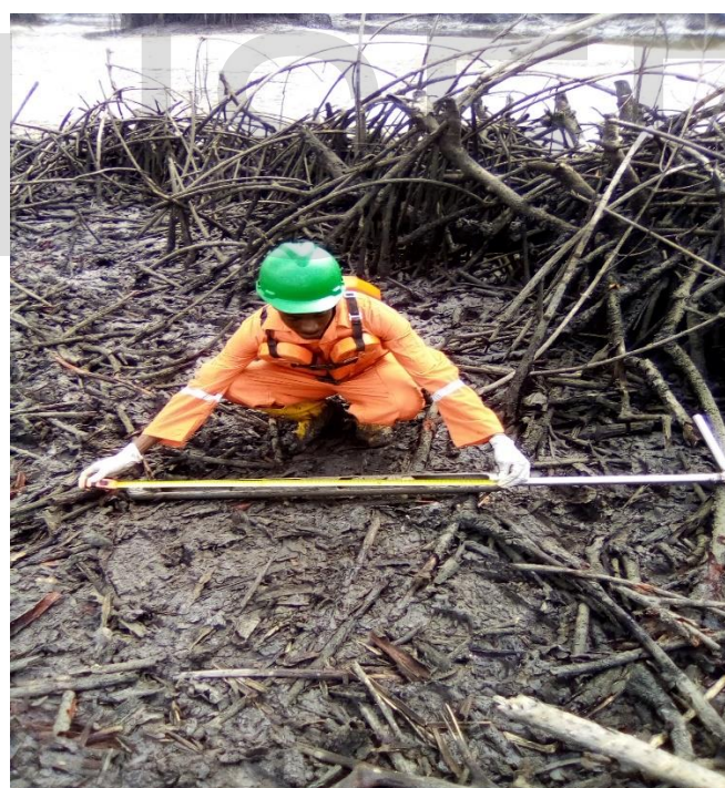
Plate 1: Sediment Sampling in the Field using Gouge Auger
